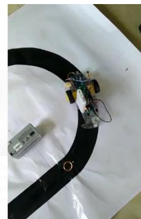
Fig -3: The cart reads the RFID tags placed on the track.
