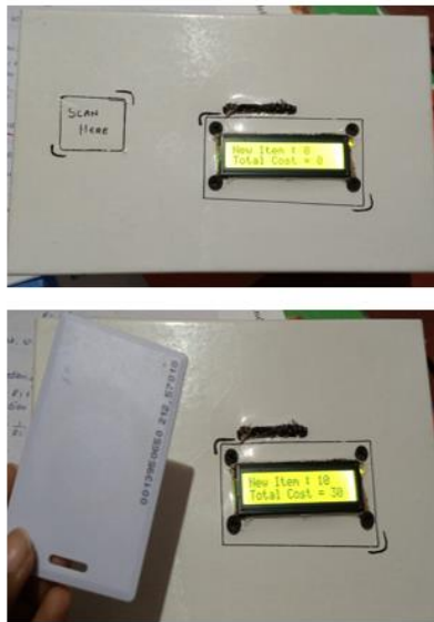
Fig -4: Each product is scanned, item's cost and total amount is displayed on the LCD screen.
