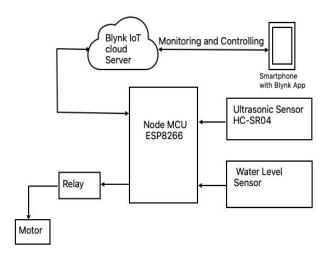
Here, we use Node MCU, which is a low cost IoT platform running on ESP8266 WiFi System on Chip(SoC). An ultrasonic sensor HC-SR04 can be used to sense the tank water level, which uses sound waves to calculate the distance as  $s=0.03430^{*}(T/2)$ , where 0.03430 is speed of sound in air in cm/microsecond and T is time taken for
