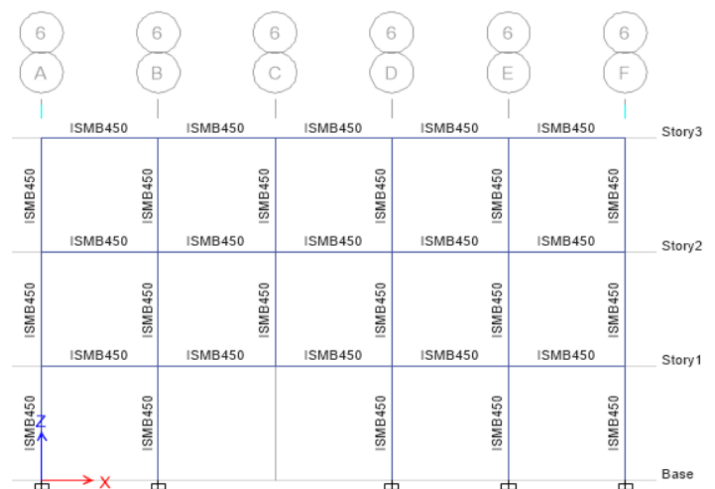
Fig -1: Elevation View of a Three Storied L Shaped Building with External Floating Column without Bracing
