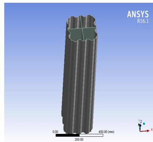
Fig. 2 Middle stiffened corrugated steel column
