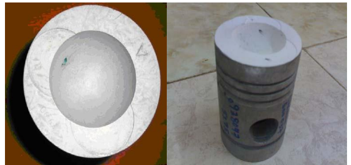
Fig 2: Photographic views of base engine and TiO 2 coated piston
