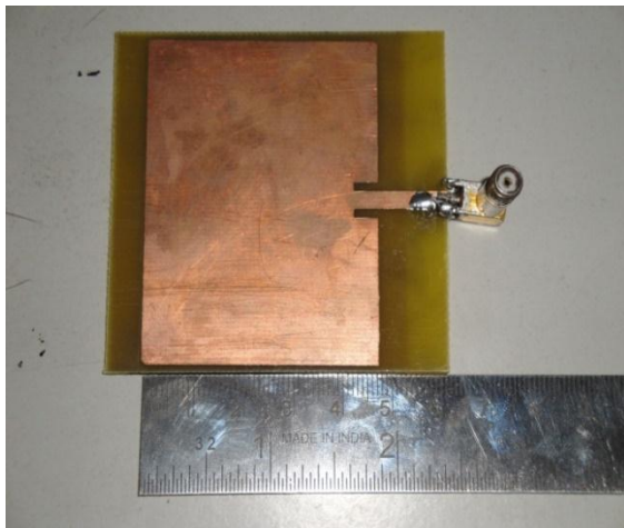
Fig-9: Photograph of Finally Fabricated Microstrip Patch Antenna Using Double C Ring (Top Layer).
