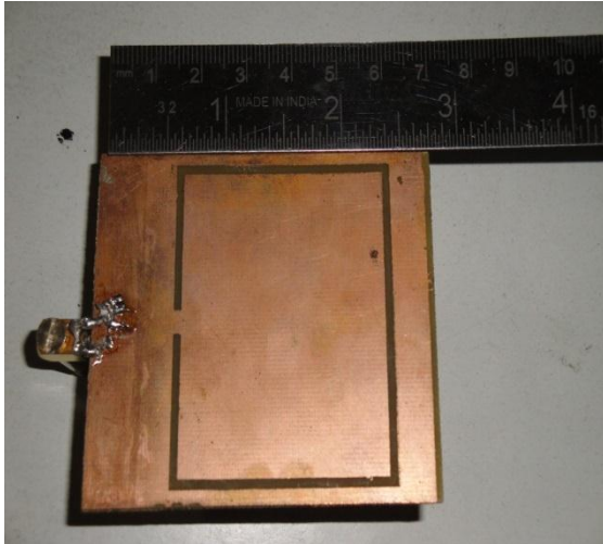
Fig- 8: PhotographOf Finally Fabricated Microstrip Patch Antenna Using Single C Ring (Ground Layer).
