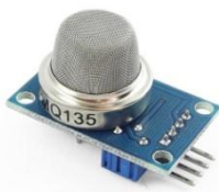
Fig – 6: Smoke Sensor
