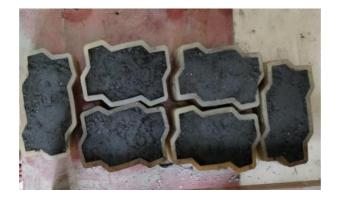
Fig. 5 – Casting of paver blocks with replacement of sugarcane bagasse ash.
