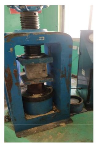
Fig. 3 – Compressive strength test of conventional concrete cubes.
