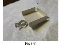
Dimensions: 100 x 90mm. The wall base is raised to 25mm, it is bent by forming. Material: Metal sheet Cost: Rs. 10 Function: This base holds the sanitizer bottle. Features: Base should be adjustable by height.
