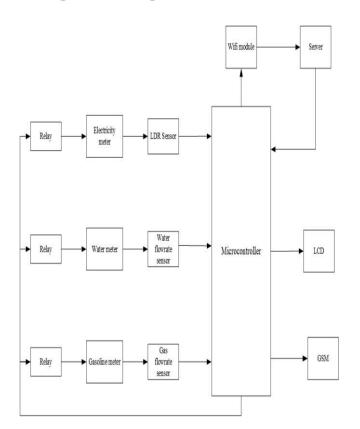
Let us consider an example for electricity consumption, here we are connecting the energy meter between main supply and load, by which microcontroller will be able to measure the energy units consumed.
