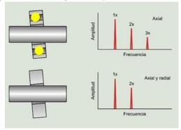
Fig -8: Bearing misalignment
