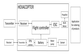
Fig 1: Block diagram of components of hexacoptor
