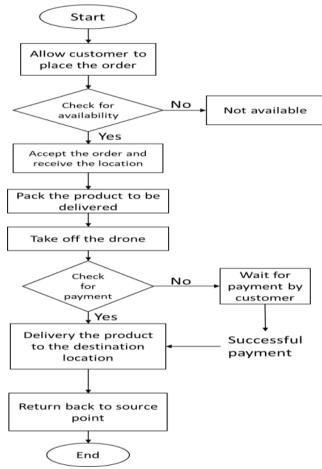
Fig 2: Flowchart of working of hexacopter
