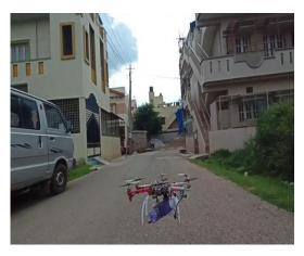
Fig 5: Hexacopter with spraying system
