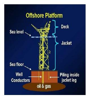
Fig 1.1: Fixed offshore platform
