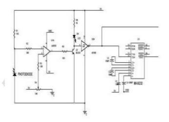
Figure 4. Laser Receiver
