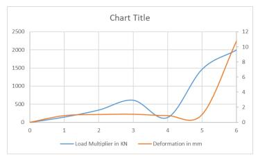
**Chart -1**: Load multiplier and deformation at 1-6 nodes
