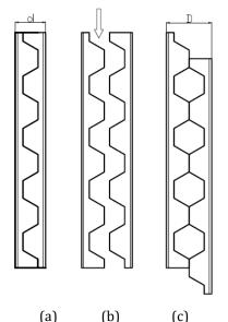
**Fig -1**: Process of castellation (a) Original ISMB with profile cutting on web post, (b) Sections after profile cutting, (c) final castellation by welding the web post.
