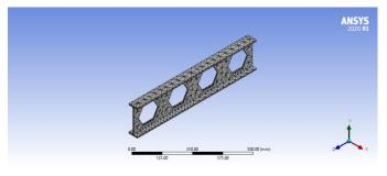
Fig -5: Meshing of Model
