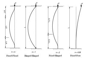
Fig -3: Different End conditions of the column
