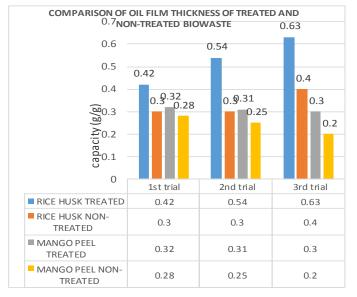
**Chart -1**: Effect of oil film thickness on the sorption capacity (g/g)
