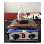
Fig 2 Pre heating of neem oil on magnetic stirrer with hot plate.
