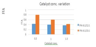
Fig 8 variation of FFA with catalyst concentration for the 6:1 molar ratio of acid catalyzed oil for base catalyzed stage of molar ratio 12:1 and 15:1
