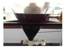
Fig 4 Separated layers after base catalyzed stage.
