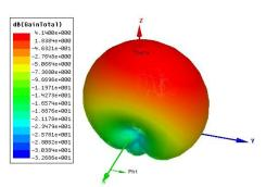
Fig 6. Simulated 2X1 microstrip patch antenna GAIN 3D (Directivity)
