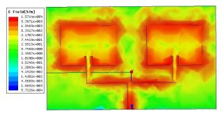
Fig 7. Simulated 2X1 microstrip patch antenna Current
