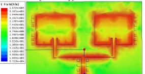
Fig 13. Simulated 2X1 microstrip patch antenna Current with EBG
