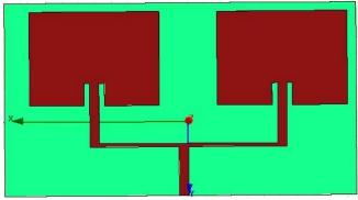
Fig1. Simulated 2X1 microstrip patch antenna design
