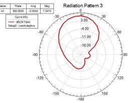
Fig 9 . Simulated 2X1 microstrip patch antenna Directivity with EBG
