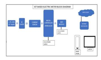
Fig -1: System Block Diagram
