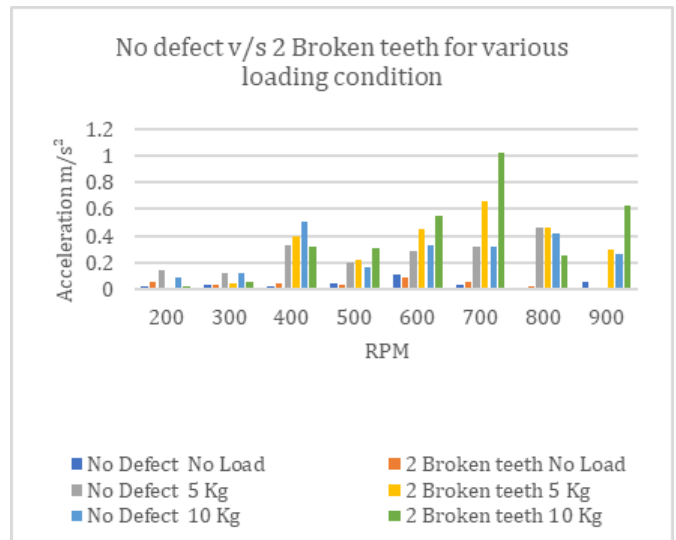
Fig -14: No defect v/s 2 broken teeth for various loading condition
