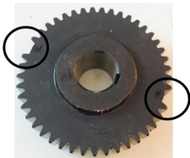
Fig -2: ADI gear with removed teeth
