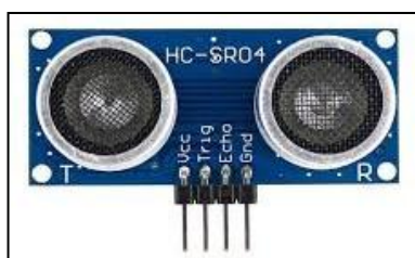
Fig. 3 : HC-SR04 Ultrasonic Sensor (source: google images)
