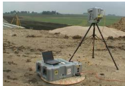
Figure 1 shows a photograph of the Cyra 2500 Laser Scanning Unit that was used in this project.
