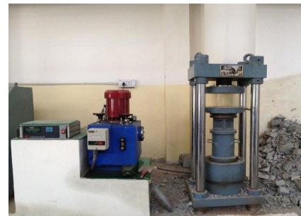
Figure-2 Compressive Testing Machine
