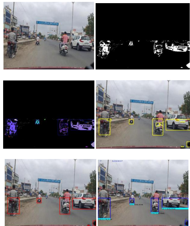
Fig -4: Intermediate stage Results (a. Original Image b. Segmentation c. Labeling d. Object Detection f. Tracking)
