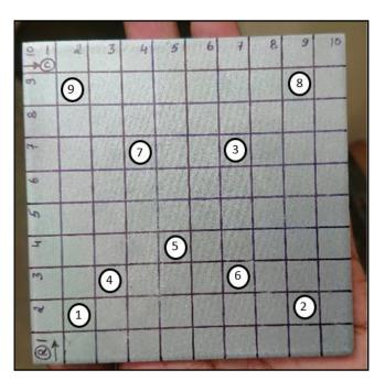
Fig-8: Random places where Hardness is measured
