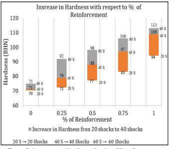
Chart-7: Increase in Hardness for % of Reinforcement.
