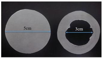
Fig-6: Diaphragm before and after it ruptures
