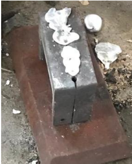
Fig: molten metal is pouring in the dies
