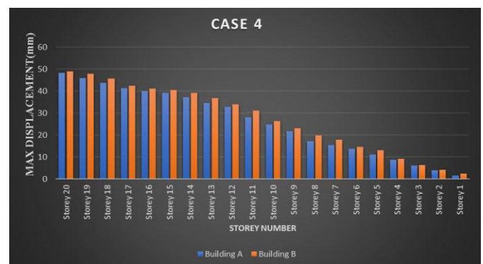
Fig -4: Displacements of Adjacent Buildings (Case 4)
