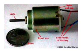
Electric motors area unit everywhere! In your house, nearly each mechanical movement that you just see around you is caused by associate degree AC (alternating current) or DC (direct current) motor. Let's begin by gazing the arrange of a straightforward two-pole DC electric motor. A straightforward motor has six elements, as shown within the diagram below:
