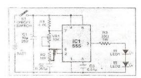
The IR transmitter half consists of Associate in Nursing below red lightweight emitting diode that may capable of causation modulated information at intervals below red band. To match the receiver frequency the into is modulated at thirty eight.7 rate by configuring 555 timer at a stable mode of operation, that generates frequency exploitation the elements
