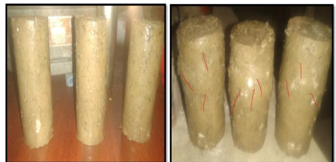
Fig -5: Cylindrical sample before load applied and afterload applied with failure.
