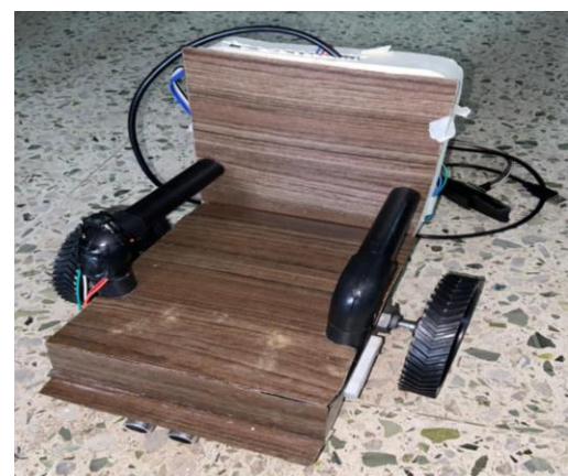
Fig -4: Final Prototype for Hand Gesture Controlled Wheelchair (1)
