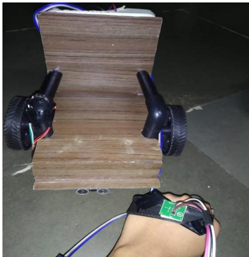
Fig -5: Final Prototype for Hand Gesture Controlled Wheelchair (2)
