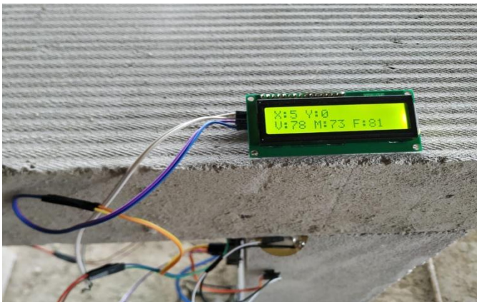
Fig -12: Implementation of 16*2 LCD and Piezoelectric Sensor
