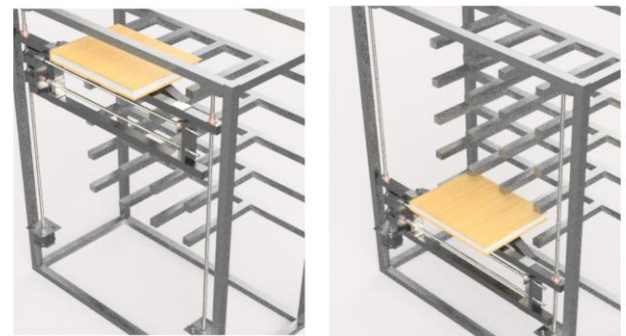
Fig -3: Differential movement of horizontal lead screw. The v-shaped structure on receiving the location of book moves to the coordinates, perform a differential motion by which they align with the book position, just below the pair of rods on which the book is placed and ensue the picking of the book.
