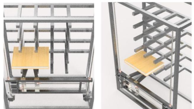
Fig -4: Book placed at the reference point. The book is brought down to the reference point and placed into the slot.
