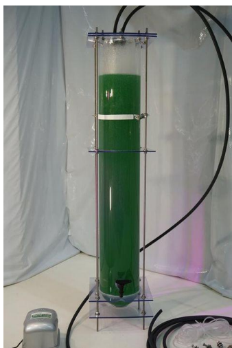
Fig.11- Closed Photobioreactor for growing Microalgae [I10]
