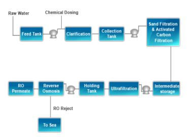
Chart -1 Typical water treatment scheme for sea water Desalination
