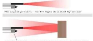
Object present - reflected IR light detected by sensor
