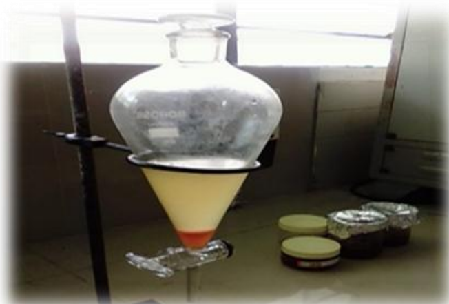
Fig - 2.3: Photographic view of obtained by-product biodiesel & glycerin in separating funnel.
