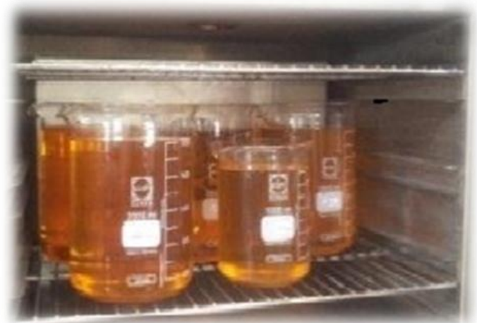
Fig - 2.1: Heating of biodiesel at 60-70 o c.
