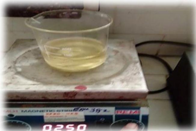
Fig - 2.2: A sample containing mixture of WCO & NaOH placed on magnetic stirrer for agitation rate at 250rpm.
