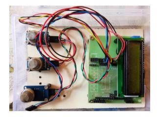
The components used in the making of prototype are Arduino board having ATMEGA 328P microcontroller and array of sensors. The analog pins of the Arduino board are connected to the Tx and Rx pins of the gas sensors. With this the measured concentration of the gas detected by the sensors can be displayed on the LED screen as well as can be displayed on the computer screen when required.
