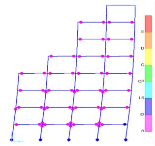
Fig- 17: Comparative location of plastic hinges at performance point (model 3)
