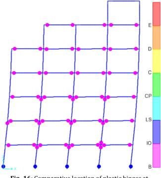
**Fig- 16**: Comparative location of plastic hinges at performance point (model 2)
