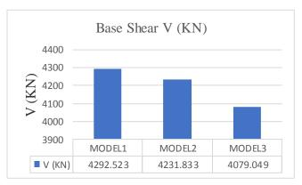
Fig-18: Comparison of base shear at performance point
