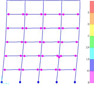
**Fig- 15**: Comparative location of plastic hinges at performance point (model 1)
