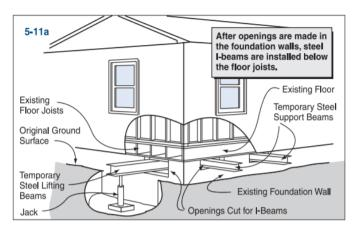
Fig. 5. Cutting holes and inserting I-Beams in foundation walls.
