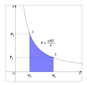
Fig 3: PV Diagram for an Isothermal process
