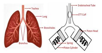
Fig 1: (a) Human respiratory system. (b) Mechanical equivalent model for an intubated patient
