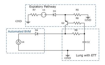
Fig 5: Equivalent electrical circuit for patient ventilator interaction
