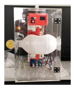
Fig 9: Prototype of Low Cost Respiration Control Device
