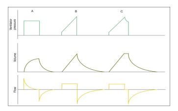
Fig 4: Human Respiration Mechanics for Different Modes of Ventilation A. Pressure Control B. Flow Control C. Volume Control
