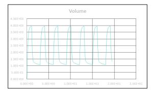
**Fig 7**: Output Capacitor Charging Profile for the Equivalent electrical circuit for patient ventilator interaction
