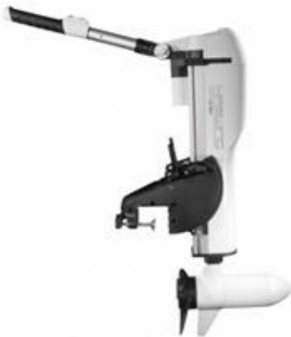
Figure 1: A typical electric Outboard propulsive leg.
