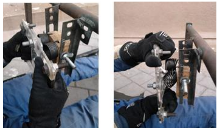
Figure 4: Use of springs to replicate steering effort
