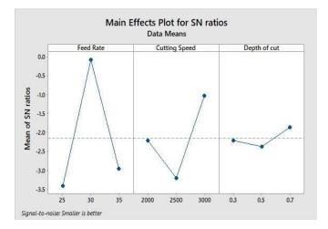
Figure 1. Effect of Feed, Speed & Depth of cut on Ra[2]
