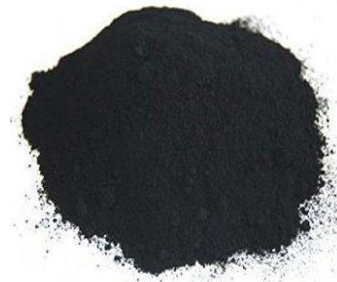
Fig -3: MoS 2 Solid lubricant powder
