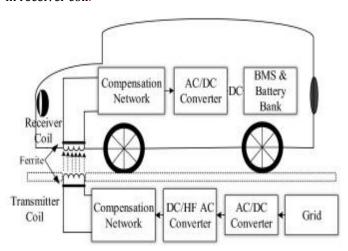
The most important thing for efficient wireless charging is to maintain the resonance frequency between transmitter coil and receiver coil so to maintain this resonant frequency compensation networks are added on both the sides. This AC power at receiver side rectified to DC through AC/DC converter and fed to the battery through Battery Management System (BMS) or Battery bank.
