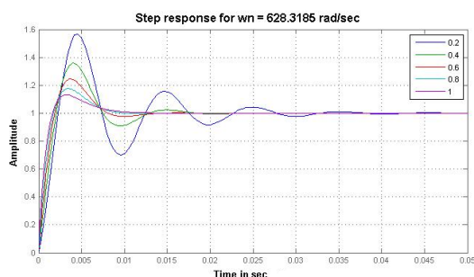
Fig.7 Step-response for \omega_n=628.3185 rad/sec and \zeta varying from 0.2 to 1
