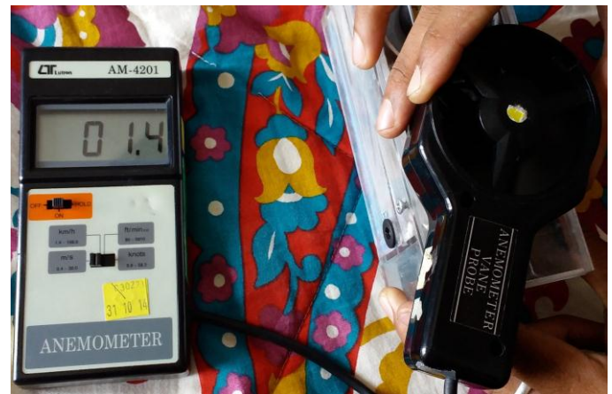
Fig -4.1: Actual outlet velocity (with loss) measured by Anemometer
