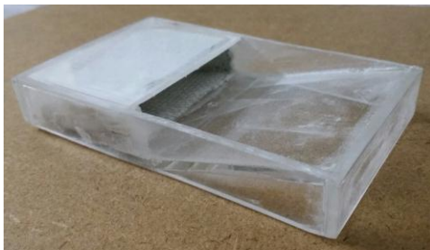
Fig -2.2: Chalk dust collecting chamber
