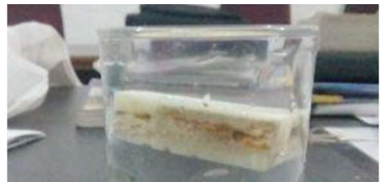
Fig-3.4: Water Absorption Test
