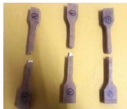
Fig-3.2: Specimen after Fracture
