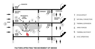
The air movement generated by mechanical ventilation will cause the pressure difference inside the building to be the same as natural forces and superimposed. By designing HVAC system which supplies air at a high rate. HVAC system is becoming now a days more and more popular for buildings. The main advantages of HVAC system limits infiltration of air which caused by winds and stack effects. Improved HVAC equipment can be linked to fire and smoke systems to overcome smoke control duties.
