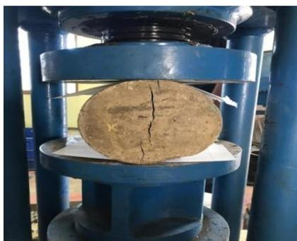
Compressive strength data were initially used to admixture-incorporated specimens to determine the optimal admixture replacement %. 3 cubes of silica fume with replacement percentages of 0%, 2.5%, 5%, 7.5%, 10%, 12.5%, and 15%, 3 cubes of fly ash with replacement percentages of 0%, 5 percent, 10%, 15%, 20 percent, 25 percent, and 30%, 10 cubes with 50% recycled aggregate replacement, and 3 cubes of rice husk ash with replacement percentages of 0%, 5%, 10%, 15%, and 20% After that, ten
